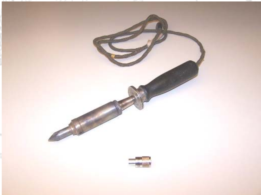
Black Beauty Soldering Iron (with a PL-259 to show scale)
