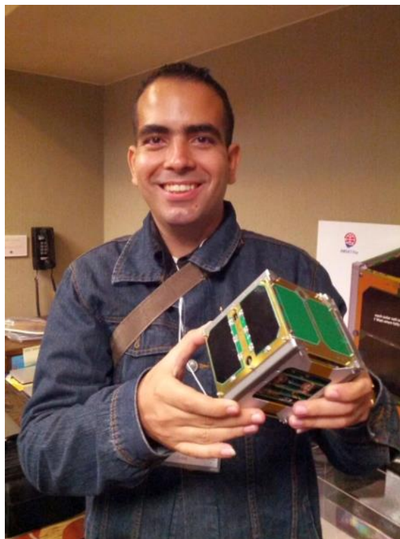
Hector Martinez CO6CBF/KF5YSV at the Symposium holding an engineering prototype of the Fox-1A cubesat. Note the size compared to the older satellites above.
