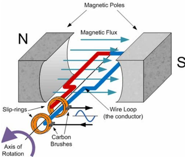
Some generators will turn at 1800 RPM. This is achieved by adding a second coil/loop on the armature. The engine is turning at half the speed as a 3600 RPM model, but creates the same number of electrical cycles with each revolution. The end result is a 60 Hz power output. Most 1800 RPM generators are diesel-fueled. Small 1800 RPM gas generators are exceptionally rare.
