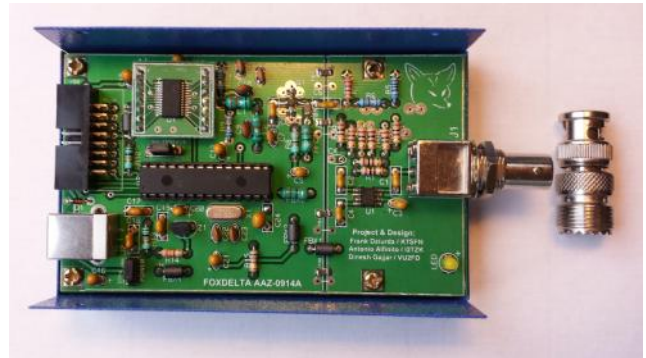
Clockwise from upper left: synthesizer daughterboard, resistor bridge, antenna connector, level detector chip, PIC microcontroller with crystal, USB connector, expansion connector.
